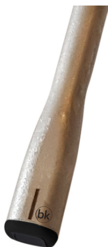
Figure 3. The orientation marker on the transducer tip.
